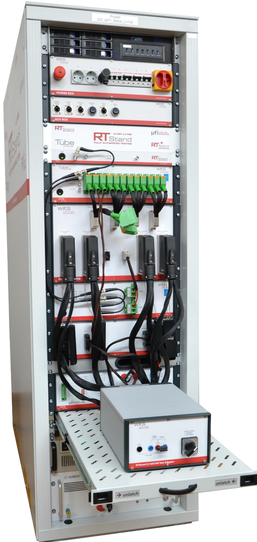
Figure 2. RTStand LV124 / LV148 fully automated testing system
